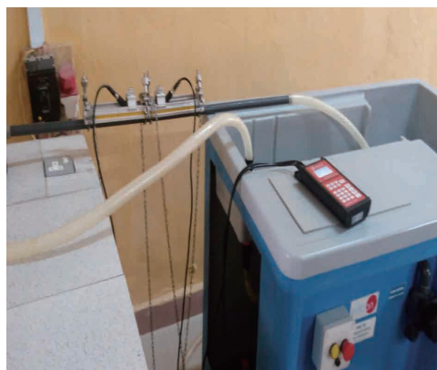
Figure 2 A set-up of V-method in the hydraulic bench
