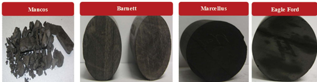
Figure 1 Mancos Samples Looked Like in Water Less Than 15 wt% NaCl or KCl, Barnett, Marcellus, and Eagle Ford Shale Samples Looked Like in Fresh Water
