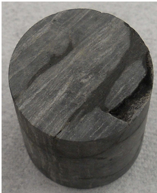
Figure 8 The Corner Was Broken Because of Generated Fractures
