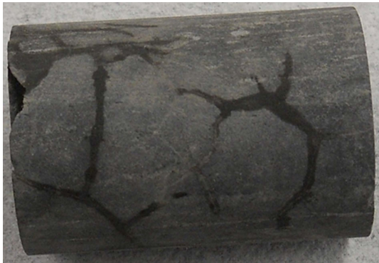
Figure 7 Dark Water Lines Showed Generated Fractures After the Core Plug Was Taken out of the Core Holder
