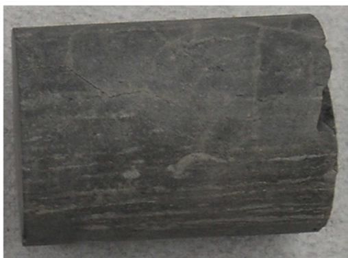
Figure 9 Fractures Remained After the Water Vaporized
