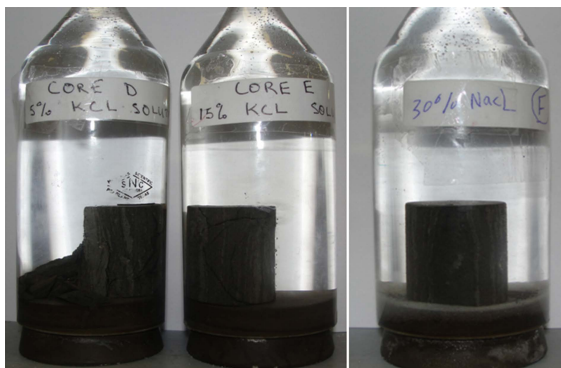
Figure 4 Mancos Samples in 5%, 15% and 30% KCl Solutions
