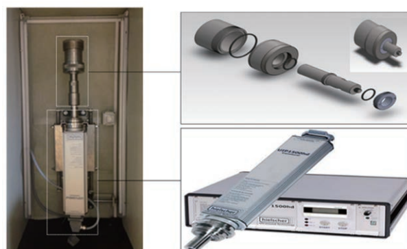
Figure 2 Ultrasonic Generator and Reactor
