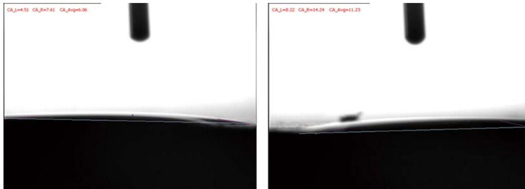
Figure 10 Results of Wettability(Contact Angle) Test of Coal Rock From Well Q2 502.89 m (After Dipped in 0.4%SLJ-2 Solution)
